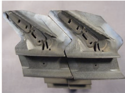
26. Conventional weld repair of HPT blade shrouds (left) looked like this after 13,000 hours of operation; upgraded extended-life repairs (right) remained “like new” after 24,000 hours
