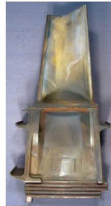
27. First-stage bucket for 7EA will be rejuvenated after 92,000 hours of service with the expectation of completing another cycle and retiring at around 116,000 hours—thereby confirming the value of extended-service-life repairs
