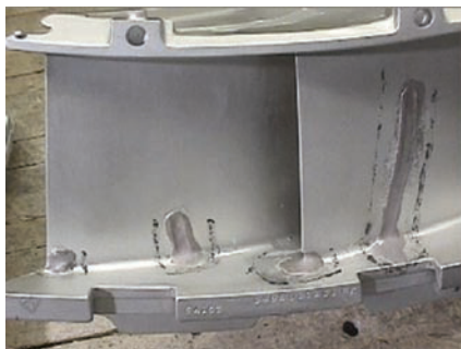
29. Nozzles after 48,000 hours of service (left) exhibit areas with large cracks. These were repaired with Liburdi’s proprietary high-strength LPM material. After 92,000 hours, areas where cracks were repaired show little re-cracking and sometimes none. LPM material can be re-repaired to further extend service life
