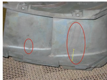
29. Nozzles after 48,000 hours of service (left) exhibit areas with large cracks. These were repaired with Liburdi’s proprietary high-strength LPM material. After 92,000 hours, areas where cracks were repaired show little re-cracking and sometimes none. LPM material can be re-repaired to further extend service life
