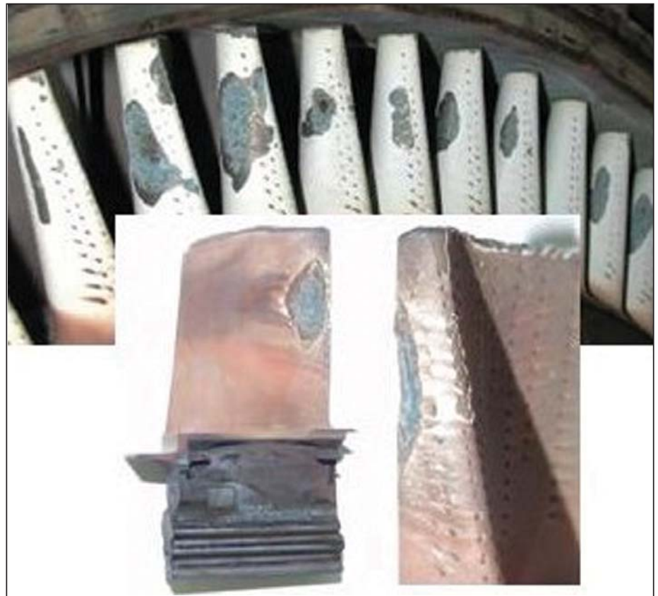
Figure 1: Water or steam injection will accelerate coating loss on stage 1 buckets due to oxidation
