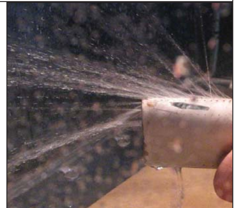
Figure 2: Spray pattern in the water flow test on the blade shows poor film cooling coverage
