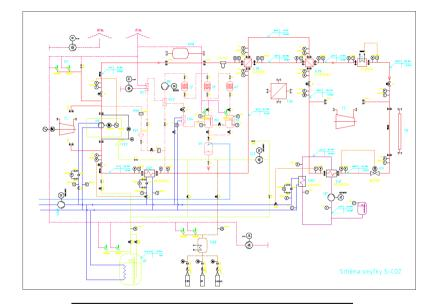
Small loop •Pressure up to 25MPa •Temperature up to 550 °C •Flow up to 12m3/hour •Power of primary pump 125kW •Electrical heating input power 500kW
